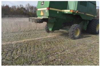
Photo 2. A chaff-lining chute concentrating weeds seeds in a narrow row during harvest, while spreading the straw and large plant residue pieces in the width of the combine header. Credit: Claudio Rubione, University of Delaware.
