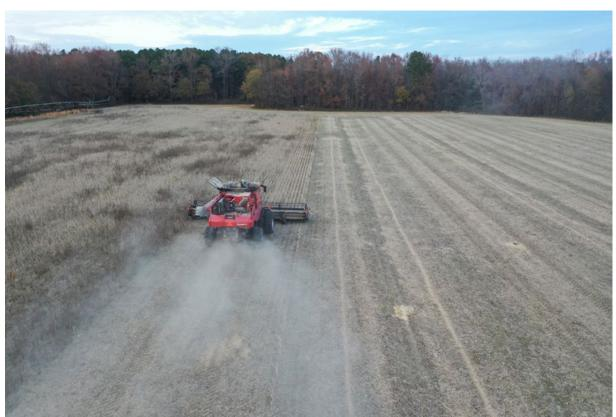
Photo 3. Combining soybeans, note the already-formed chaff lines next to the combine made with a fabricated chute. Credit: Claudio Rubione, University of Delaware.
